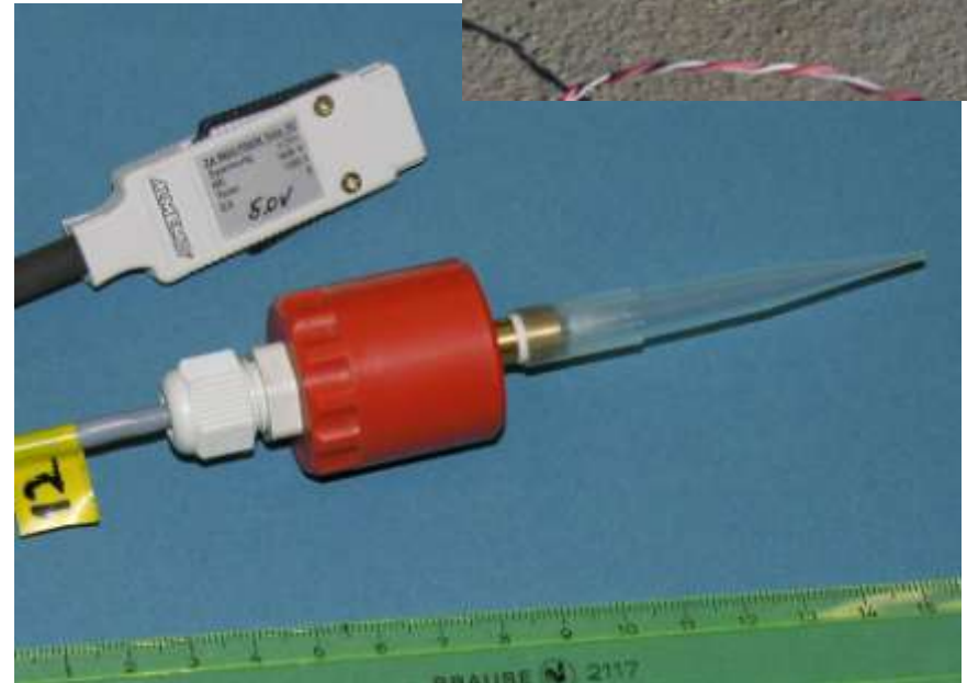
Capillary pressure measurement (construction site)
