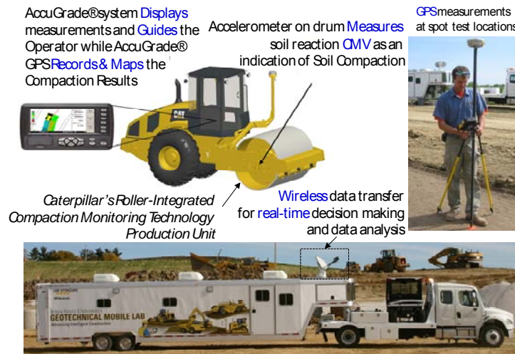
Figure 1. Compaction monitoring technology with display system (upper left), GPS measurement using hand-held rover to link machine measurements with in-situ test locations for correlation analysis (upper right), and mobile geotechnical laboratory for rapid field testing and wireless data transfer (bottom).
