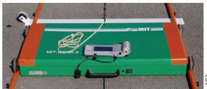
A closeup of the MIT Scan-2 resting on a new concrete pavement.
