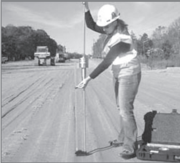
Figure 6B—One person One person operates DCP, then marks the tape on the Vertical Scale.
