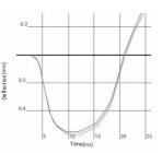
Test on insufficiently compacted soil. Individual deflections strongly decreasing with significant differences between single drops. E<sub>vd</sub> value below possible optimum, s/v > 3.5.
