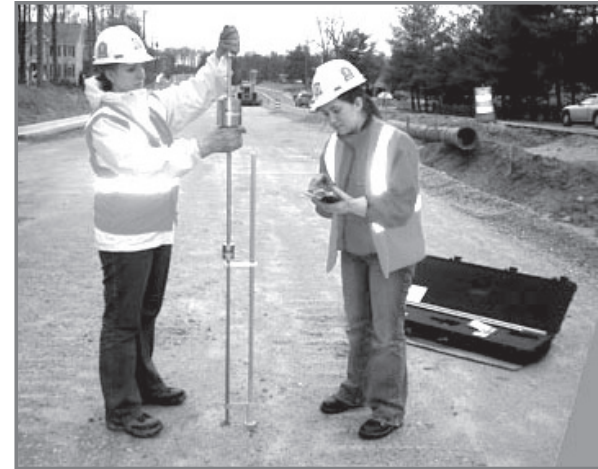
Figure 6A –Two person, traditional method One person operates DCP while the other person records penetration rate
