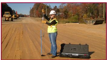
DCP Model K100AD is strong, compact and ergonomically designed for use at Airfields for evaluating subgrades below pavements.
