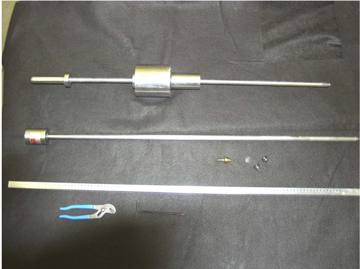
FIGURE 1 Picture of the U.S. Army Corps of Engineers (USACE) Dual Mass DCP
